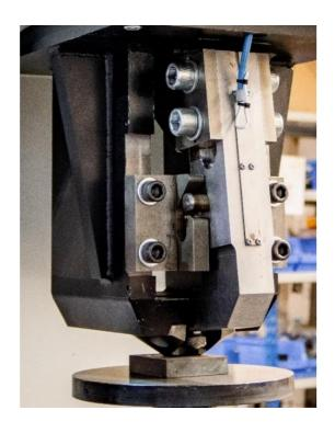
Helios test head during bench trials, with covers removed to show heavy-duty construction and machine strength. This test head has been continuously refined and remains the industry benchmark for heavy-duty applications.
