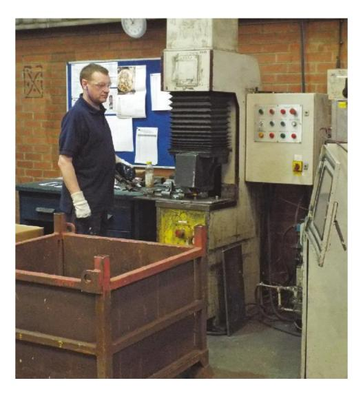
One example of the BRINscan Mk III tested every link in every tank track used by the British Army over a 35-year period, with only one breakdown, ever. The machine was still working flawlessly when 'retired' as a precaution.
