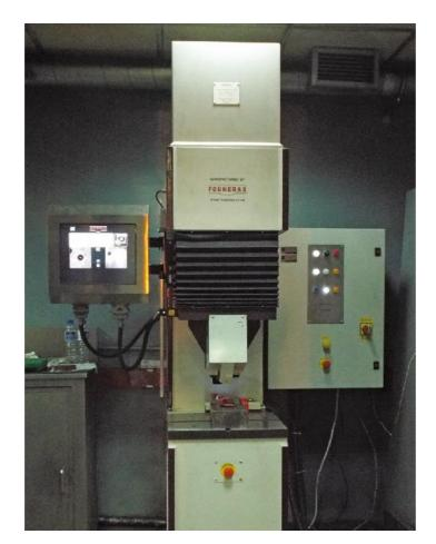
The latest generation of the BRINscan range, the MKV Brinell hardness tester, offers fully automatic indentation measurement and recording of test results and is built for the toughest of heavy-duty industrial applications.
