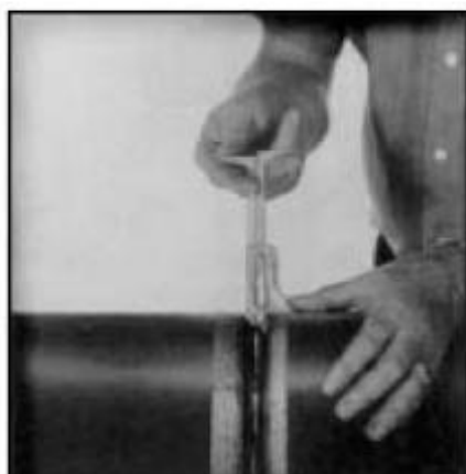
Measure internal mismatch, pipe wall.
