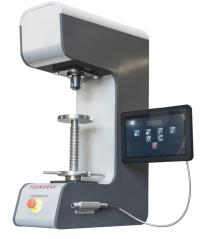
The Robus D incorporates an automatic Brinell measurement unit. This supremely accurate system significantly exceeds the requirements of the standards, and operator error is virtually eliminated. Indentation measurement (reporting to 4 decimal places) takes a matter of seconds.
