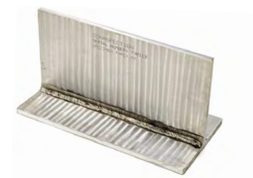
An example of a magnetic testing tee specimen
